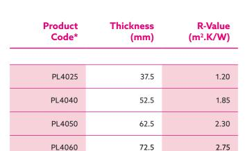
\*Last three digits of product code are thickness of insulation in mm. Total thickness includes additional 12.5mm plasterboard.
