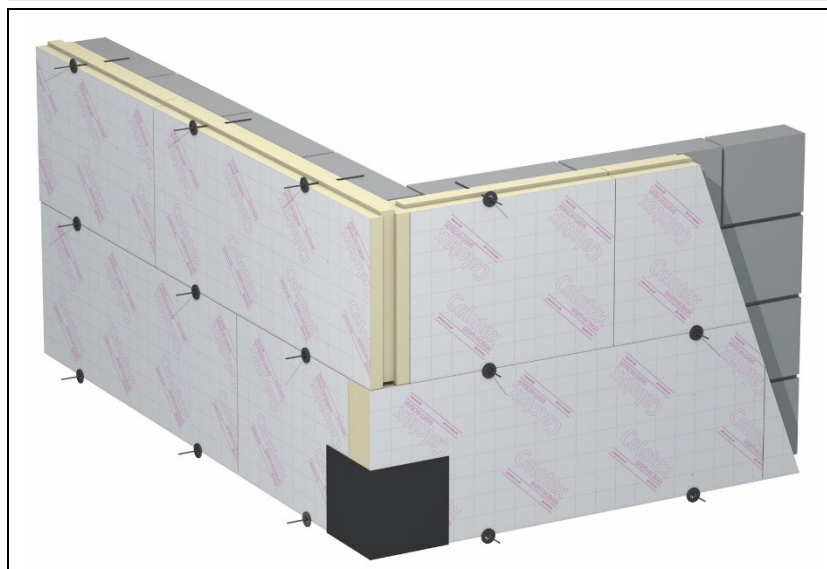
Figure 5 Corner board blocking arrangement
